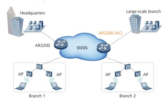
The AR2200 routers integrate AC (Access Controller) functionality, which can manage the wireless AP (Access Point) in wireless LAN. AR2200 supports rich certification and flexible user access control, which can provide security access guarantee for Wi-Fi users. The rich wireless capabilities integrated in one device, this can realize centralized management of wired and wireless networks, to meet the requirements of different scale enterprises networks.
