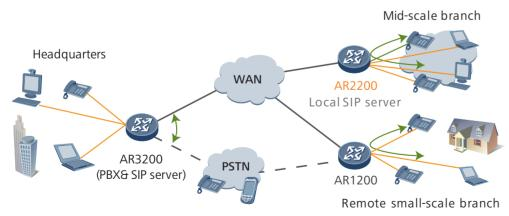
To improve communication efficiency, all AR routers include built-in PBX. This feature supports the enterprise main number, Interactive Voice Response (IVR), and bill query functions. An AR1200 router can provide intelligent dialing in a smaller branch office.
