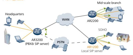
To enhance the corporate image and improve communication efficiency, all AR routers include a built-in PBX. This feature supports the enterprise main number, Interactive Voice Response (IVR), and bill query functions. The AR1200 can also be located in a branch office to provide intelligent dialing.
